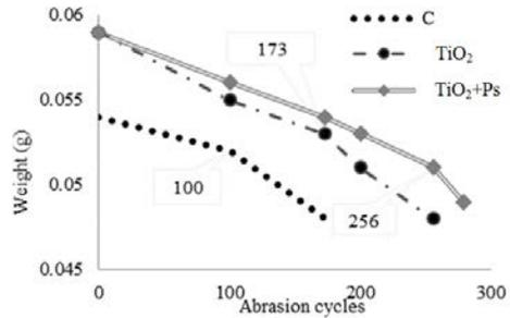
FIGURE 6. The weight reduction versus number of rub cycles.
