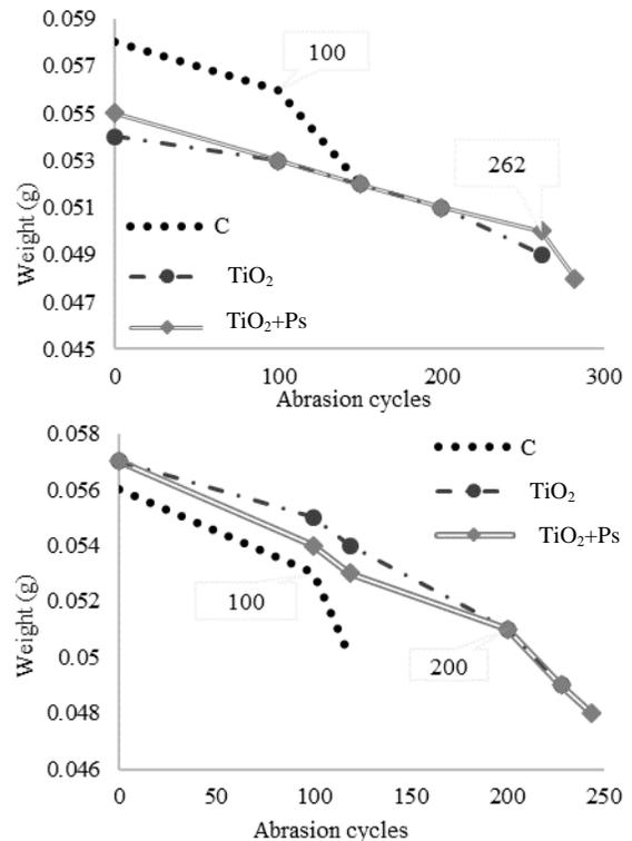
FIGURE 7. The weight reduction versus number of rub cycles after a) 100 h and b) 160 h UV irradiation.
