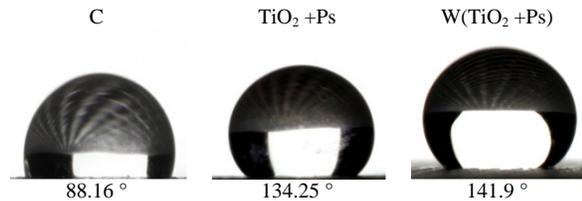
FIGURE 2. Contact Angle (CA) on different samples.
