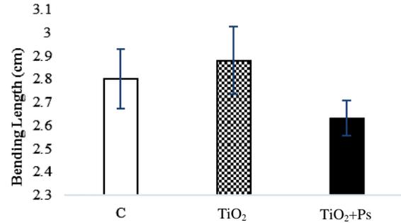
FIGURE 3. Bending length of different samples.
