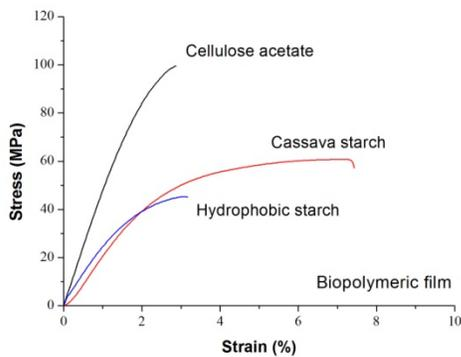
FIGURE 8. Typical stress-strain behavior of biopolymeric films.
