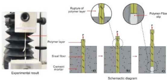
FIGURE 12. Schematic pull out behavior of treated fiber.
