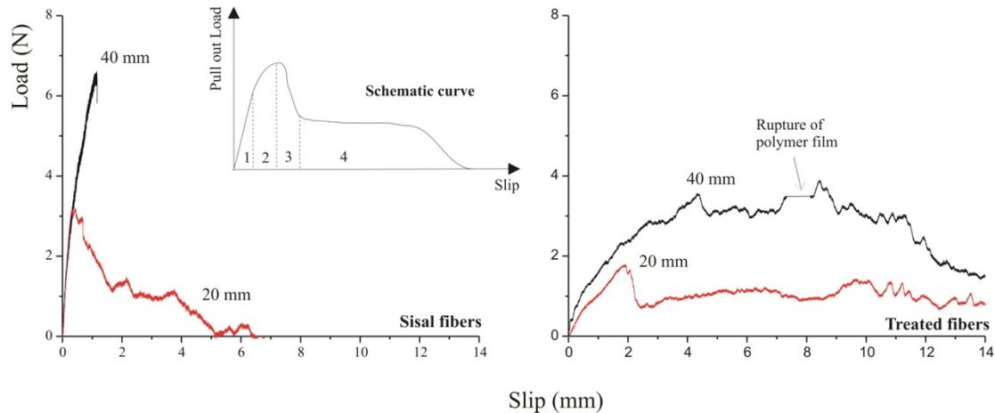
FIGURE 11. Tension-pull out curves of natural sisal fibers and treated (CA treatment) in cement matrix.
