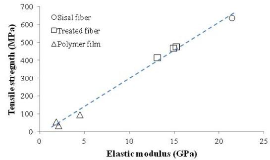
FIGURE 10. Correlation between mechanical properties for untreated fiber, film and treated fiber.
