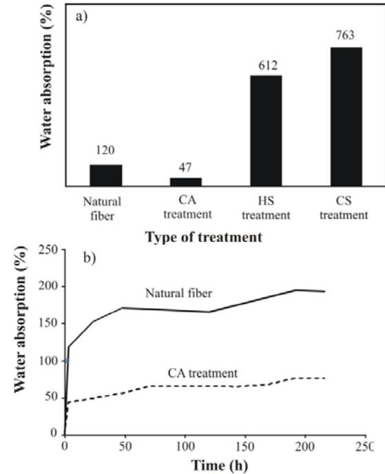
FIGURE 7. Effect of treatment on water absorption of sisal fiber after : a) 3h; b) 9 days.
