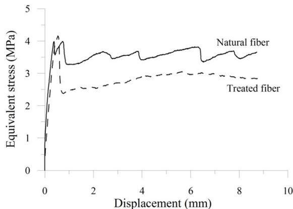
FIGURE 13. Effect of fiber treatment on the flexural behavior of sisal fiber cement composite.
