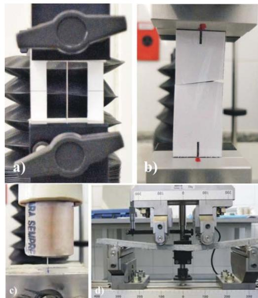
FIGURE 3. Test setup: a) tension of fiber; b) tension of film; c) pull out; d) flexural of composite
