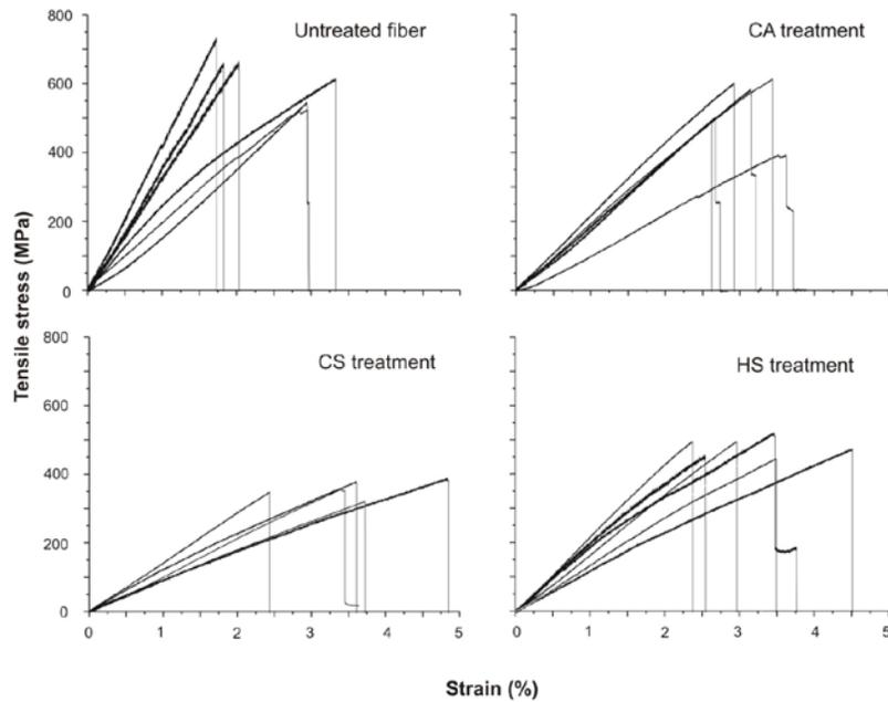
FIGURE 9. Effect of treatment on stress-strain behavior of sisal fiber.
