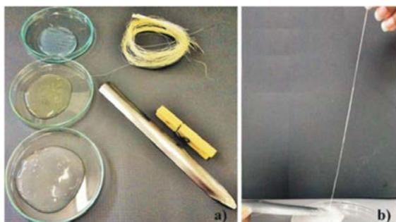
FIGURE 2. Treatment of fiber: a) biopolymeric gels; b) immersion of fiber.
