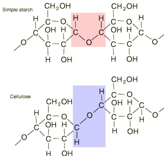
FIGURE 1. Structural formulas of starch and cellulose [36].
