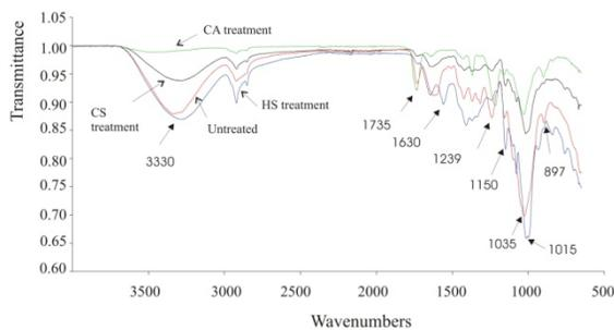
FIGURE 6. Fourier transform infrared (FTIR) spectrum for treated and untreated sisal fiber.
