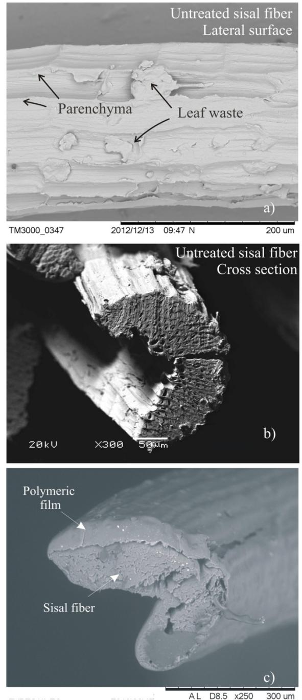
FIGURE 4. Effect of treatment on surface texture of sisal fiber: a,b) untreated fiber; b) treated fiber.
