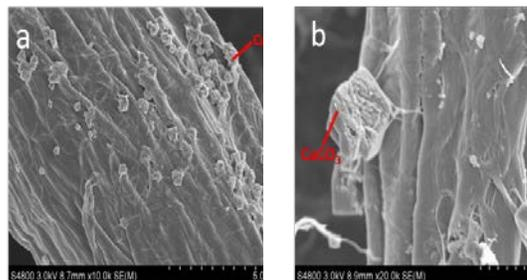
FIGURE 2. The SEM images of the cellulose/ $\text{CaCO}_3$  fibers.
