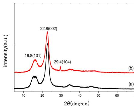
FIGURE 3. XRD patterns of (a) native softwood chemical pulp fiber, (b) cellulose/ $\text{CaCO}_3$  modified fiber.
