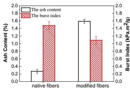
FIGURE 4. The burst index of the pulp.
