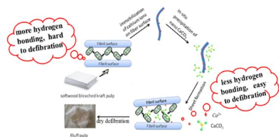
FIGURE 1. Schematic of the concept of preparing the cellulose/CaCO<sub>3</sub> modified fibers for enhanced the defibration process of fluff pulp.
