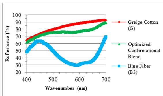
FIGURE 5. UV-Vis Spectra of greige control (IV) fiber (red), optimized fiber blend from the confirmation experiment (green), and the blue-dyed (III) fiber (blue).
