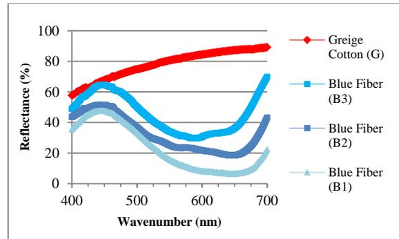
FIGURE 3. Comparison of UV-Vis spectra of Greige Cotton (G) and blue-dyed fibers (B1, B2, B3).
