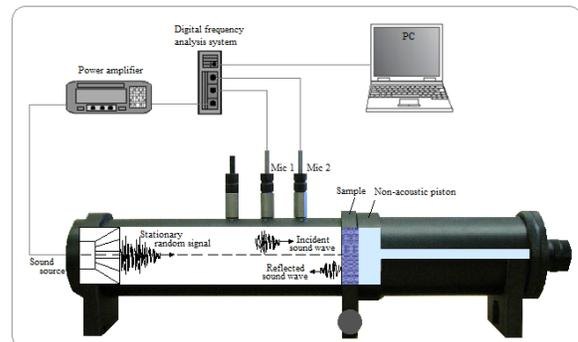
FIGURE 3. Schematic diagram of impedance tube and measurement devices (Adapted from Brüel & Kjær Sound & Vibration Measurement A/S) [16].
