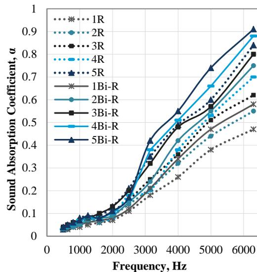
FIGURE 6. Sound absorption of T and Bi-T samples.
