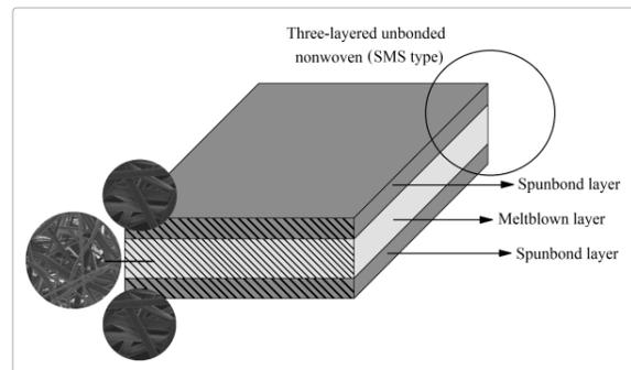
FIGURE 1. Fabric design of multilayer nonwovens.
