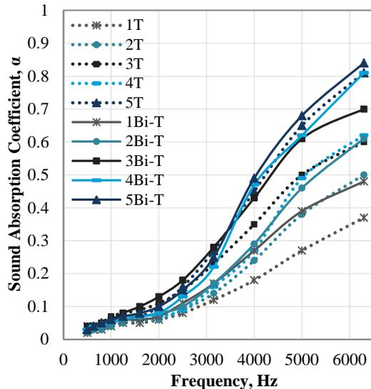
FIGURE 7. Sound absorption of T and Bi-T samples.
