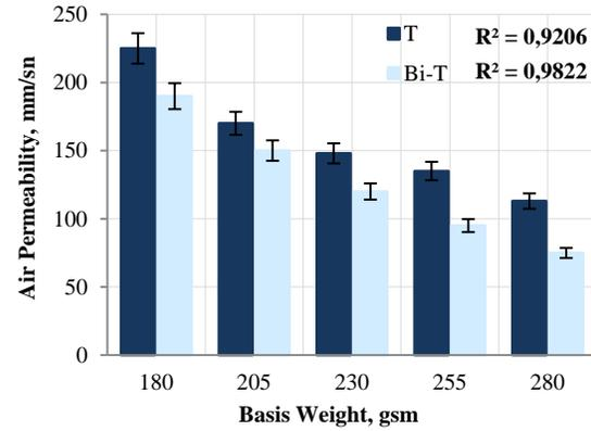
FIGURE 5. Air permeability of T and Bi-T samples.
