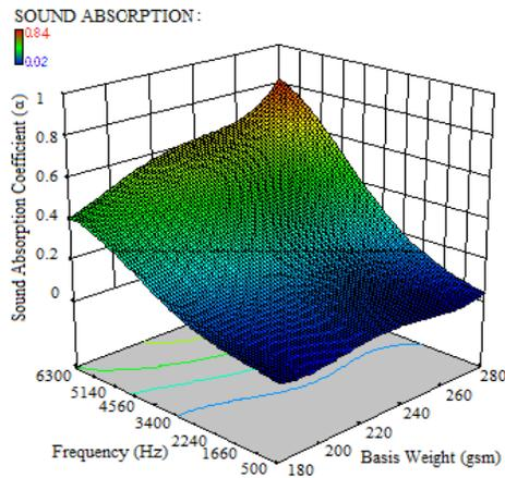
FIGURE 8. Interactive effects of basis weight and frequency on sound absorption coefficient for R and T samples.
