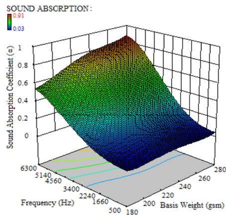
FIGURE 9. Interactive effects of fabric weight and frequency on sound absorption coefficient for Bi-R and Bi-T samples.
