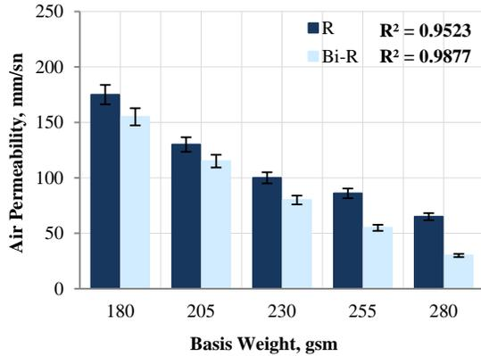
FIGURE 4. Air permeability of R and Bi-R samples.
