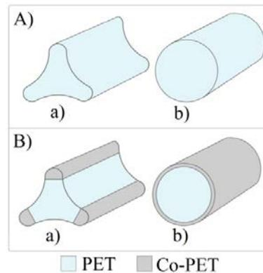
FIGURE 2. Fiber Cross-sections; A)Homocomponent fibers; a)Trilobal, b)Round; B)Bicomponent fibers; a)Bico-trilobal, Tipped trilobal type, b)Bico-round, Core/sheath type.
