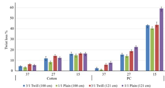
FIGURE 1. Twist loss percentage in different weft yarns.
