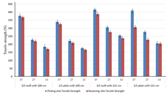
2FIGURE 6. PC Fabric weft wise tensile strength.
