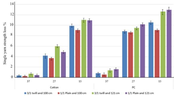
1FIGURE 4. Single yarn strength loss percentage in different yarns.
