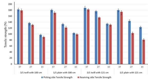
FIGURE 5. Cotton fabric weft wise tensile strength.
