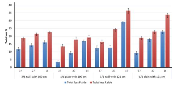
FIGURE 3. Twist lost percentage on picking and receiving side for PC weft yarns.
