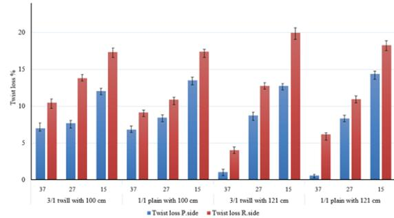
FIGURE 2. Twist lost percentage on picking and receiving side for cotton weft yarns.
