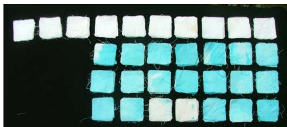
FIGURE 11. Quaternary dyeing of 3ATAC on cotton. 1 st Row: Control, APJET, NCAPS, Q, QD, QM, QP, QDM, QDP, QDMP 2 nd Row (all treated on APJET): Q, QD, QM, QP, QDM, QDP, QDMP 3 rd Row (all treated on NCAPS, dry): Q, QD, QM, QP, QDM, QDP, QDMP 4 th Row (all treated on NCAPS, wet): Q, QD, QM, QP, QDM, QDP, QDMP
