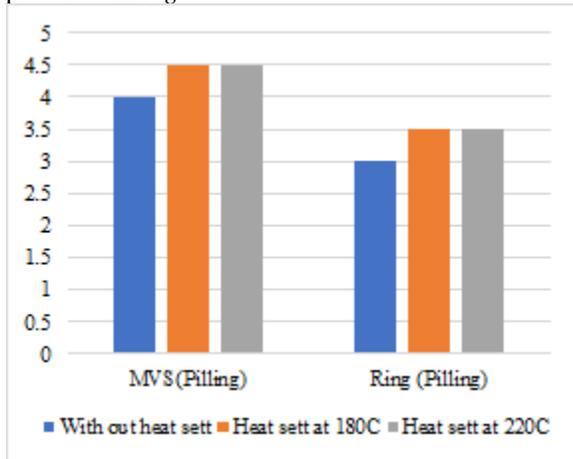
FIGURE 5. Pilling results of Pad Thermosol dyed fabric.
