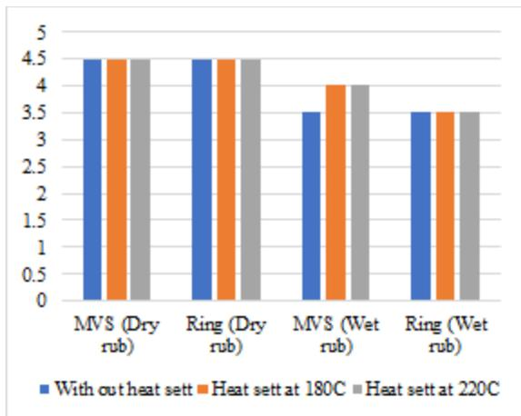
FIGURE 7. Rubbing Fastness results of Pad Thermosol dyed fabric.
