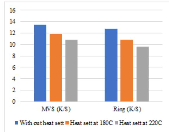
FIGURE 3. K/S results of Pad Thermosol dyed fabric.
