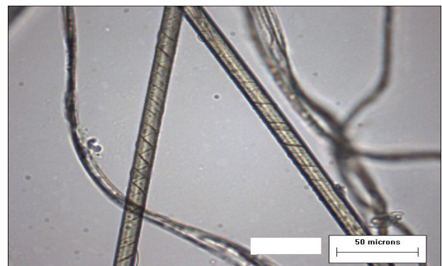
FIGURE 11. Typical fibers from para-aramid filament sewing thread CF3
