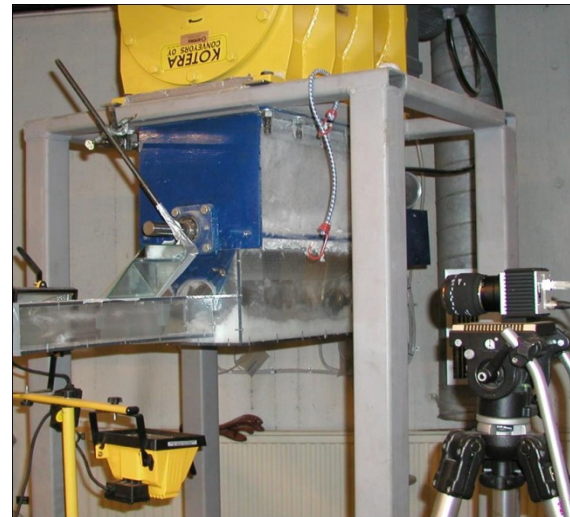
FIGURE 2. Camera setup at imaging location 1 right after the dispersator.
