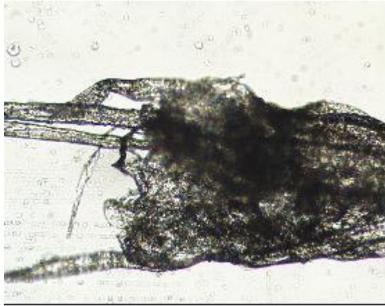
FIGURE 4. Incomplete frayed fiber cut
