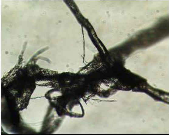
FIGURE 11. Frayed point comprised of tow fibers
