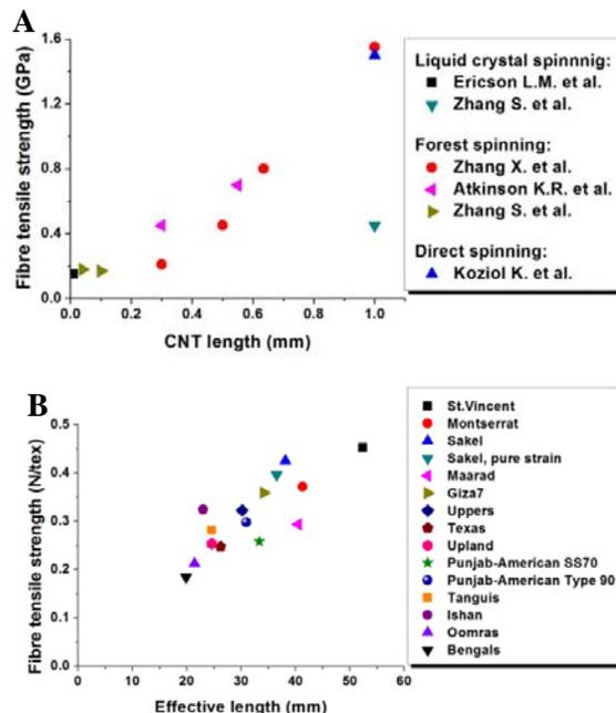
FIGURE 5. Plots of fiber strength against building block length for CNT fibers (top) and different cotton varieties (bottom). Note that the top plot is in GPa and the bottom in N/tex, as the values reported are in these units [18].
