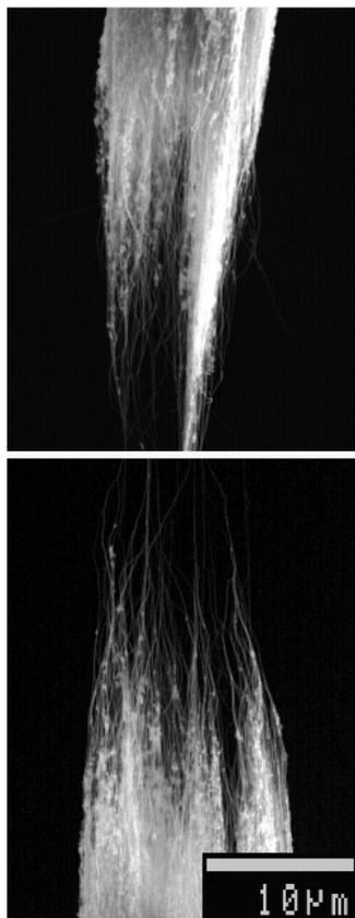
FIGURE 4. SEM micrograph of the fracture ends of a CNT fiber.
