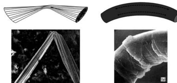
FIGURE 3. Cross-sectional change in CNT fiber with yarn-like structure (left) contrasted against 'solid' aramid fiber with evidence of kink damage due to compressive stresses due to bending (right). Aramid image from reference [16].
