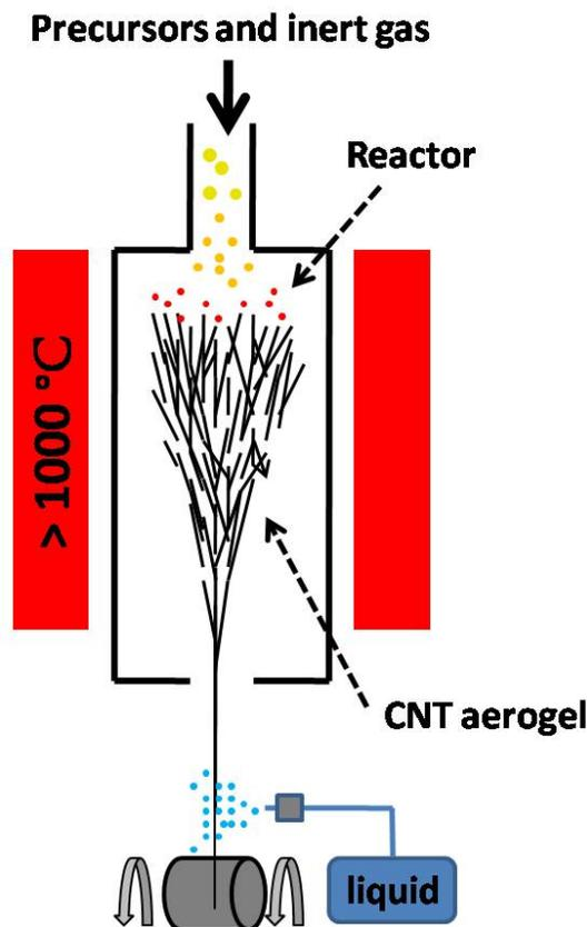
FIGURE 2. Schematic of the process for spinning CNT fibers directly from the gas-phase.
